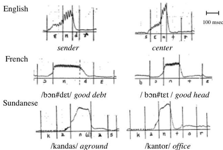
Figure 3: Filtered nasal airflow for one representative token of ND (left) and NT (right) for English, French, and Sundanese.
