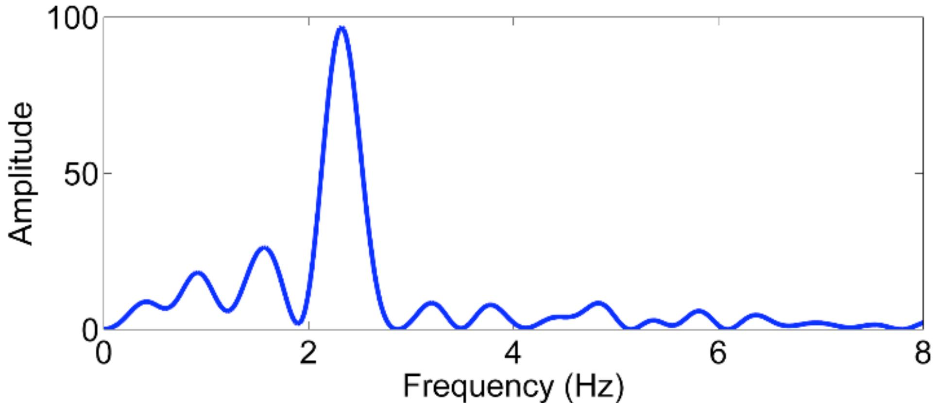
Figure 2. Fourier transform of the amplitude envelope shown in figure 1 - the “rhythm spectrum”. The peak at 2.3 Hz indicates a component with a period of about 435 ms (compare this to the interval durations in figure 1).
