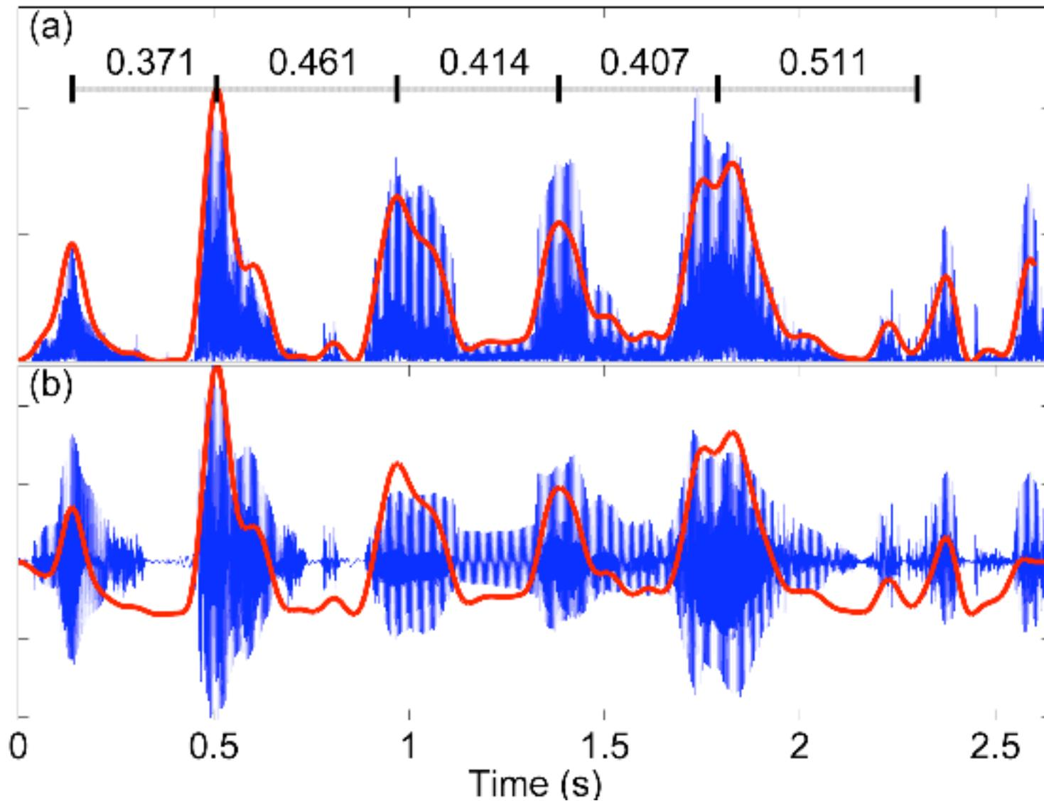
Figure 1. Taking the amplitude envelope of a 2.5 sec. stretch of speech - “at least based on money raised it looks like..”. (a) rectified signal with envelope. (b) original signal with windowed envelope. [Listen to this utterance.]
